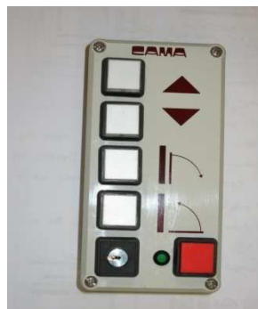
photograph shows wall mounted call-station
